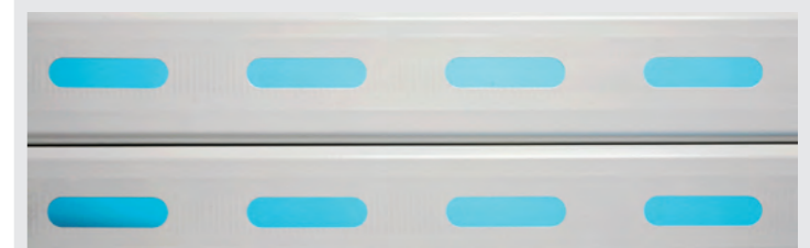
OVAL SLOTTED - Optional 25mm x 100mm Oval slotted shutter slats are available on request. Slots are spaced 65mm apart. Doors may be fully slotted or partially slotted.
