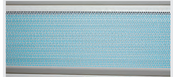
PERFORATED OPTION - Optional 3mm perforated shutter slats are available on request. Perforation is 90mm high and seen full length of slat. Doors may be fully perforated or partially perforated.
